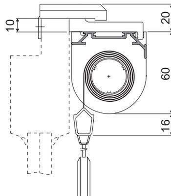
Mounting in the window jamb (with face fix bracket 33 mm)
