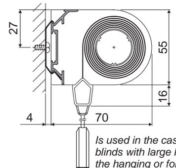
*Is used in the case of roller blinds with large heights of the hanging or for fabrics of greater thickness.*
