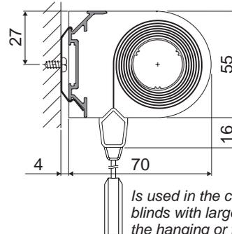
*Is used in the case of roller blinds with large heights of the hanging or for fabrics of greater thickness.*
