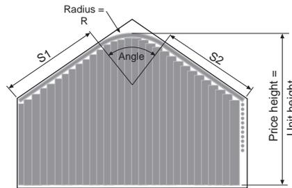
$$S1 + \text{Straightened length} + S2 = \text{Price width} = \text{Straightened track length}$$
