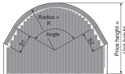
$$S1 + \text{Straightened length } R + S2 = \text{Price width} = \text{Straightened track length}$$
