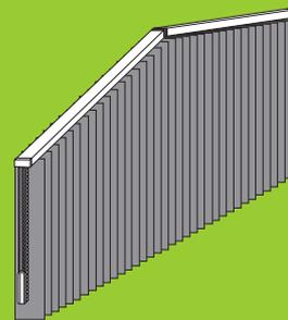
Two slope units with louvre overlap. Operation elements are fitted at the outer ends.
